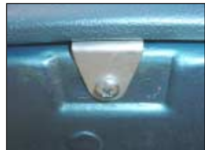
Installed panel clip
